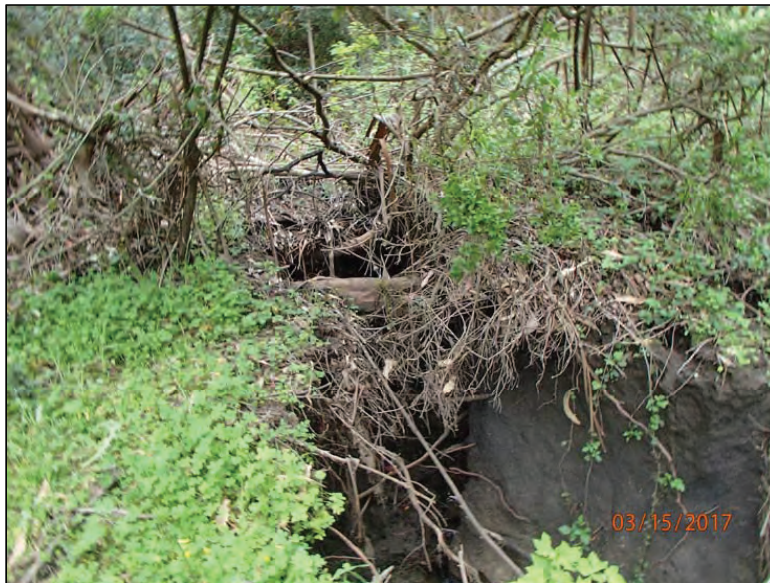
Photo 10 (Site #2): View of an active 5.5ft tall headcut at the downstream extent of the inundated pond at stream crossing Site #2 on the Meadow trail shown in the previous photo.
